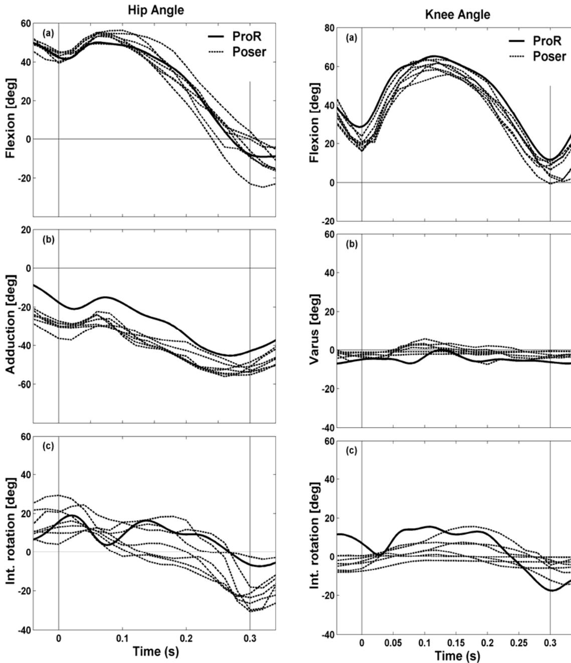
**Figure 15** Hip and knee joint angles ( $^{\circ}$ ) of the support leg, calculated with the Pro Reflex system (solid lines) and the model-matching technique for each of the seven side-step cutting matchings (dotted lines). The vertical lines indicate initial ground contact of the support leg and toe-off.
