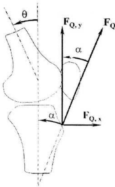
**Figure 8** From DeMorat et al. (2004) Definition of patella tendon tibial shaft angle ( $\theta$ ), knee flexion angle ( $\alpha$ ), and the anterior shear force vector ( $F_{Q,x}$ ) is the total quadriceps muscle force applied to the patella tendon.
