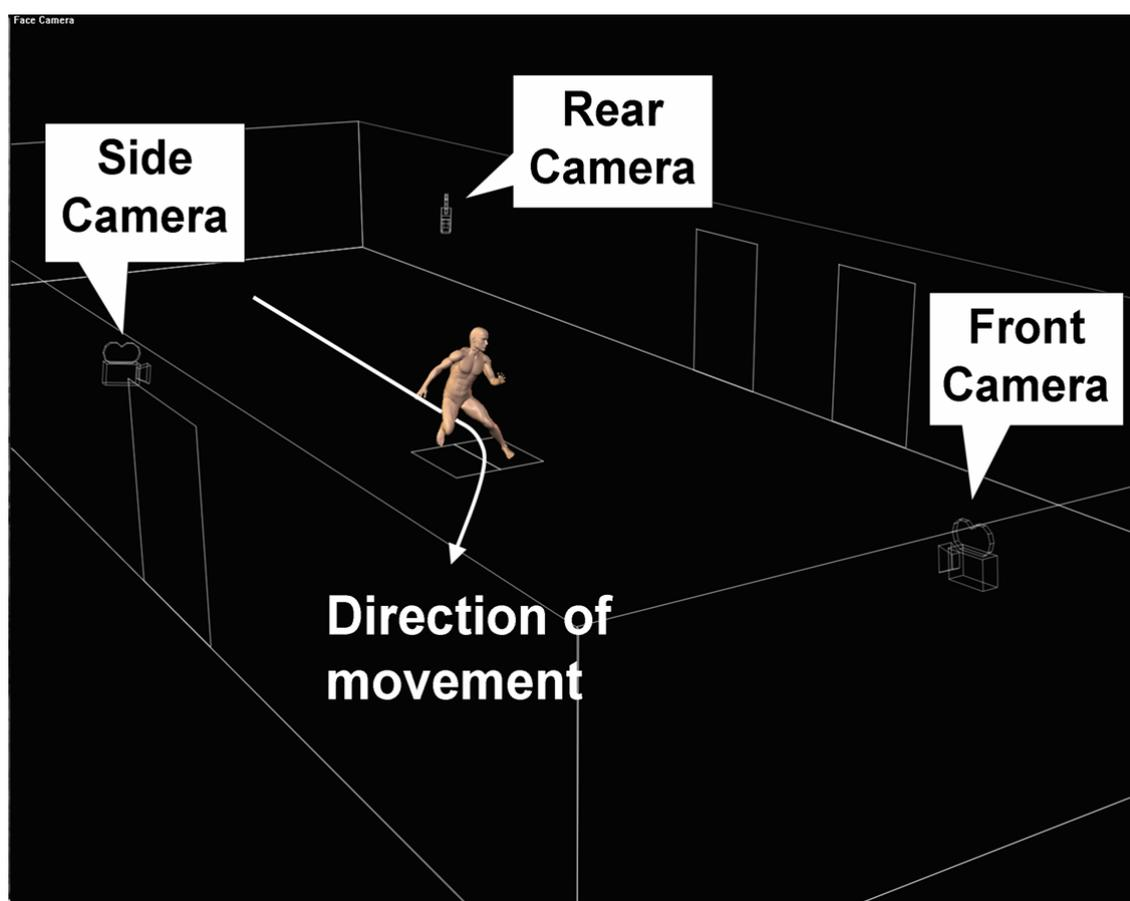
**Figure 11** Overview of the video camera placement in relation to the test subject.
